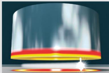
A burning ARC is put into rotation in a controlled way. A ring-shaped weld pool is generated where the welding element is plunged in.
